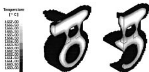
Figure 5 The temperature distribution in the tooth crown when the whole casting was 70% solidified: Design 1.
